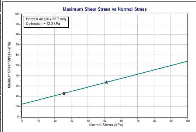
If there is more than one test result plotted, in the Maximum Shear Stress vs Normal Stress graph a line is fitted to the test results and the Friction Angle and Cohesion are calculated. The [graph options](#) <sup>[1476]</sup> are set in the template.
